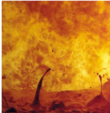
2 Oxygen blowing and addition of pellets and fluxes
